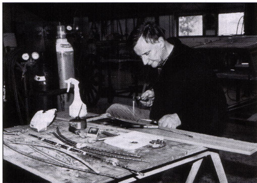
Piet Stolk solders the pins into the beading, which will be later electroplated and then varnished after being "nailed" back onto the caleche body. (Photo courtesy of Firma Stolk)
