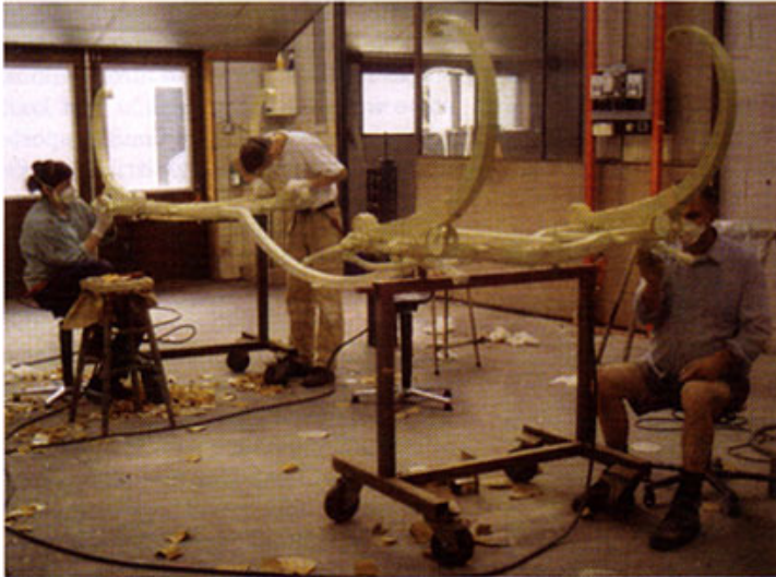
Facing a long, painstaking task, the Stolks sand the gear of the Crème Caleche in preparation for repainting and gilding. The lion's head finials require an infinite amount of patience.
